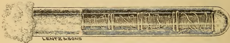
Ignition Tube containing Glass Reels wound with Silk, etc.
